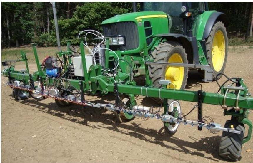
Figure 8. The experimental rig as set up for the field trials in the onion crop in the 2011 cropping season. Note the new nozzle/valve assembly design (in orange) fitted to the two booms on the far side of the machine and nozzle/valve assemblies from the previous project (in blue) fitted to the nearside boom.
