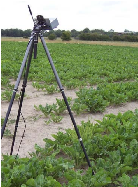
Figure 9. Stereo camera specially constructed to take stereo images of tall weeds such as weed beet
