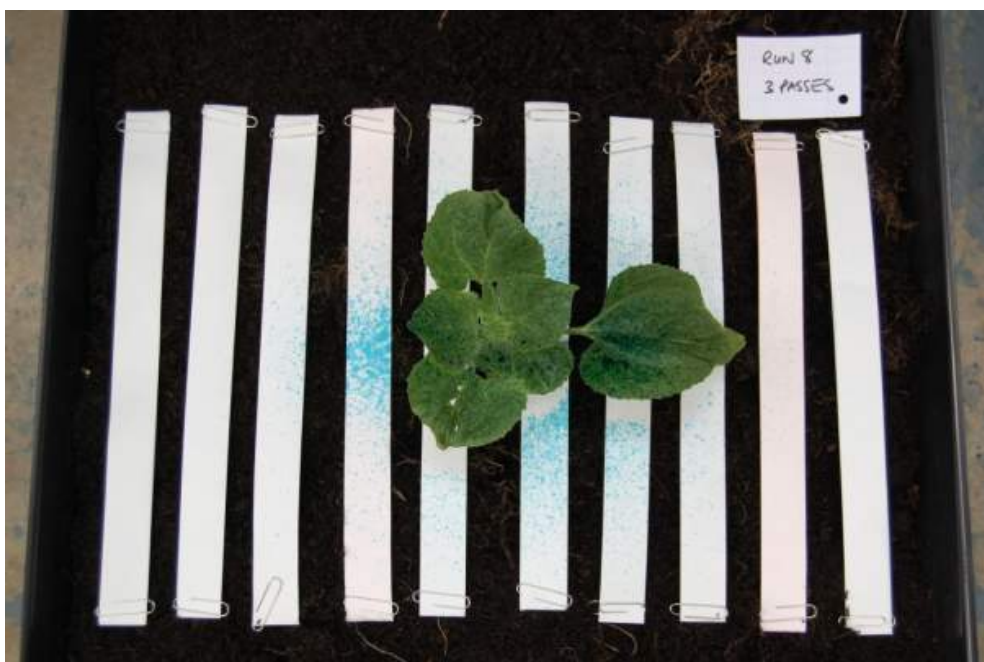
Figure 2. Dye deposits monitored on a plant surface treated with the “Even-Spray” nozzle operating 400 mm above the target, at a pressure of 3.00 bar and travelling at a speed of 4.0 km/h in still air conditions. (Note: The larger footprint compared with the “Alternator” nozzle and little evidence of secondary splash from treated leaves).
