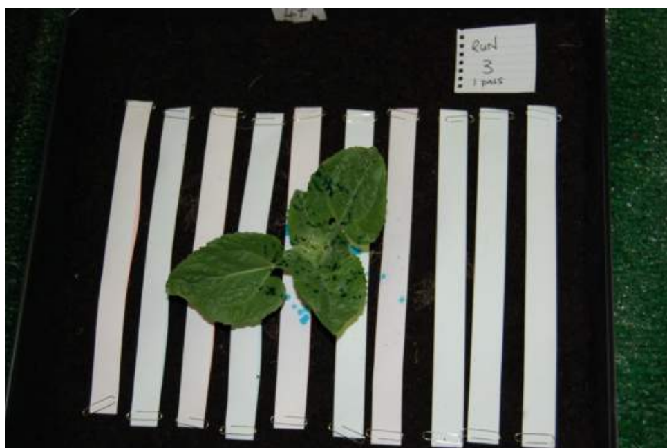
Figure 1. Dye deposits monitored on a plant surface treated with the “Alternator” nozzle operating 400 mm above the target, at a pressure of 0.75 bar and travelling at a speed of 4.0 km/h in still air conditions. (Note: Little evidence of secondary splash from treated leaves).
